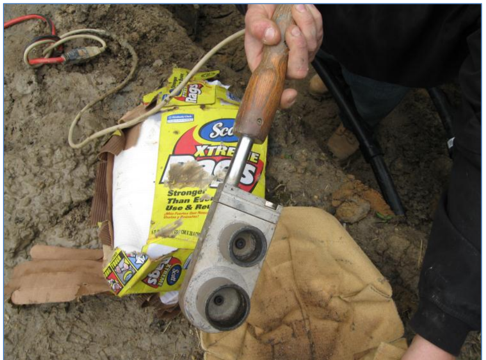
Photo: 23: Here's a close-up of the iron used to thermally fusing loop pieces together;
