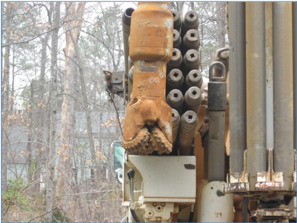
Photo 8: Close-up of one of the rotary drill bits; and stock of 20ft. drill pipe sections;
