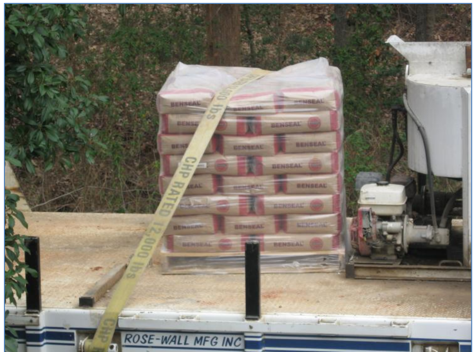
Photo: 19: Bags of bentonite clay on top of a service truck that accompanied the drilling rig; the hopper on the right is used to mix the clay powder with water before pumping it into the boring;
