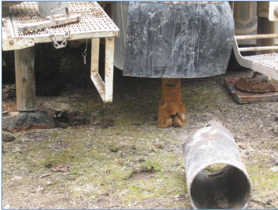
Photo: 9: Rotary bit positioned to begin drilling;
